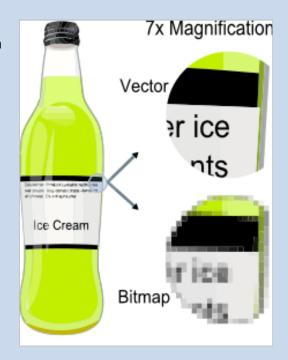
Computer displays are made up from grids of small rectangular cells called pixels; the term comes from "picture elements". The picture is built up from these cells. The smaller and closer the cells are together, the better the quality (resolution) of the image, but a larger file is required to store the increased pixel count. However, modern storage devices and working memory have gigabyte, even terabyte capacities, so there is less need for particularly compact forms of data.
